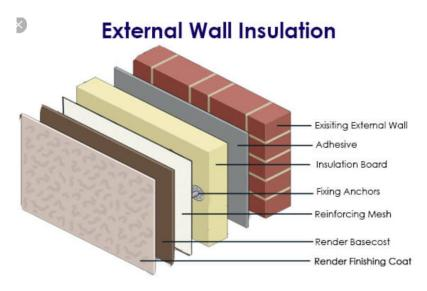
Suitable fixings are available from any regular building merchant and it's recommended that the insulation fixings should be at least 110mm long to ensure they go through the insulation to the brickwork.
